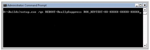
The location of the setup.exe file will depend on where on the system the Creator install files are located.
