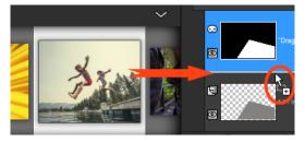
It's important to drag the image thumbnail under the blackand-white mask layer. The pointer displays a plus sign and a line displays between the layers to indicate that you are inserting an image layer.
