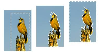
You can create a selection by using a Selection tool shape (left), by creating a freehand selection (center), or by using the Magic Wand tool to select specific areas of color or opacity (right).
